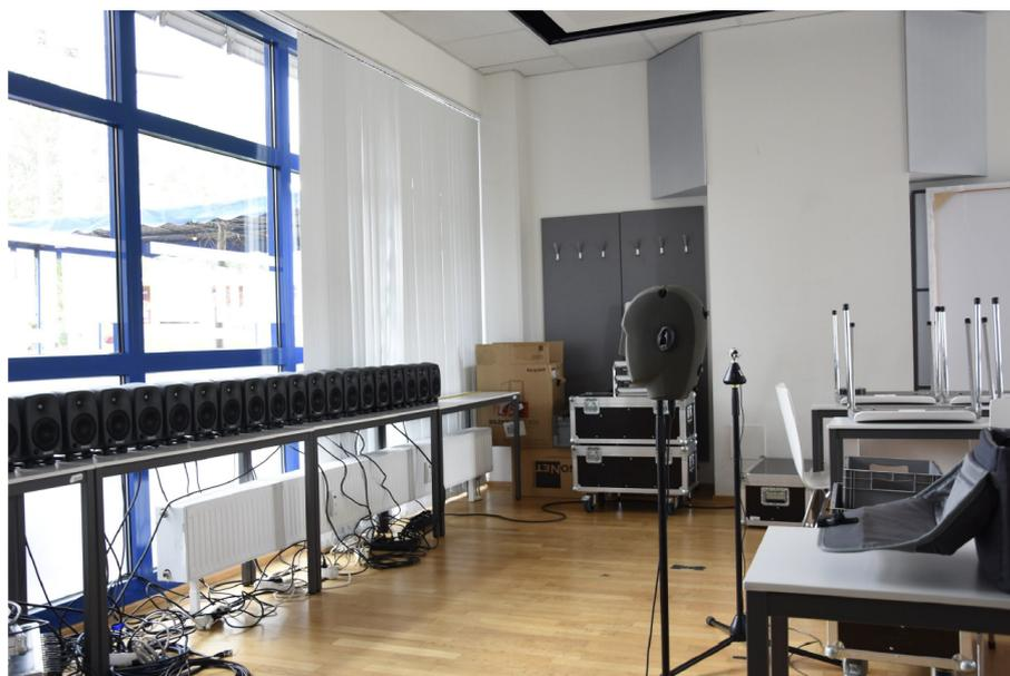
Figure 10: Setup for recording binaural impulse responses
