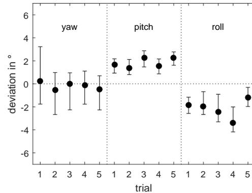
**Fig. 5:** Median and interquartile range of the error propagation for the BNO055 based tracker for *Yaw*, *Pitch* and *Roll* rotation in five continuous trials.
