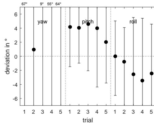
**Fig. 6:** Median and interquartile range of the error propagation for the GY-85 based tracker for *Yaw*, *Pitch* and *Roll* rotation in five continuous trials.
