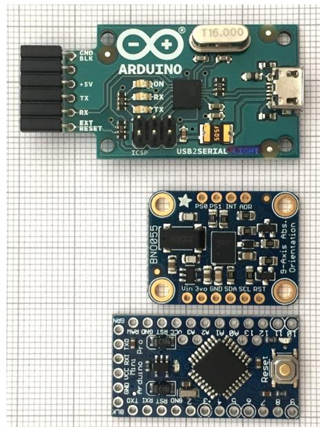
**Fig. 2:** Used components of the *MrHeadTracker*. Top-down: Arduino USB2Serial (24x42 mm, without connectors), Adafruit BNO055 (20x27 mm), Arduino Mini (18x33 mm).
