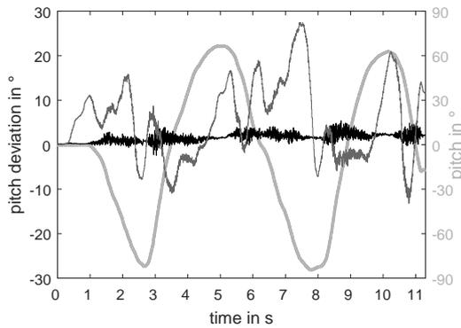
**Fig. 4:** Pitch deviations of the BNO055 based head-tracker (black line) and GY-85 based head-tracker (thin grey line) compared to the trace of the optical reference system (thick grey line).
