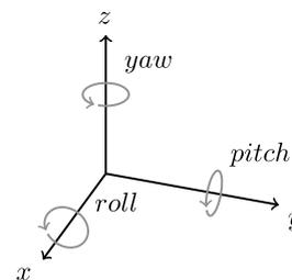
Fig. 3: *Yaw*, *Pitch* and *Roll* movements [5].
