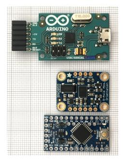
Fig. 2: Used components of the *MrHeadTracker*. Topdown: Arduino USB2Serial (24x42 mm, without connectors), Adafruit BNO055 (20x27 mm), Arduino Mini (18x33 mm).
