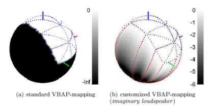
Figure 6: Visualization of the effect of the imaginary loudspeaker [4].
