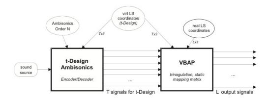
Figure 7: Block schema of the presented hybrid approach. The round windows state initializations where the cartesian coordinates of the loudspeakers are in matrix form of  $T \times 3$  and  $L \times 3$ .
