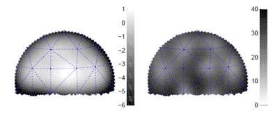
Figure 9: Ambisonics: The total signal power E (left) in dB and the angular spread measure  $\sigma_E$  (right) in degree for a virtual t-design using L=180 loudspeakers and the order N = 4 [4].
