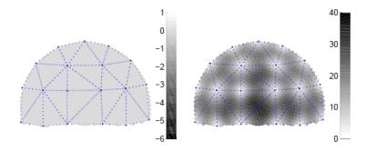
Figure 8: VBAP: The total signal power E (left) and the angular spread measure  $\sigma_E$  (right) for a sample triangulation. [4].
