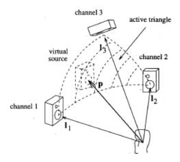
Figure 5: Three-dimensional setup of loudspeakers. A phantom source is created inside the area of the triplet by playing back coherent signals with different amplitudes [3].
