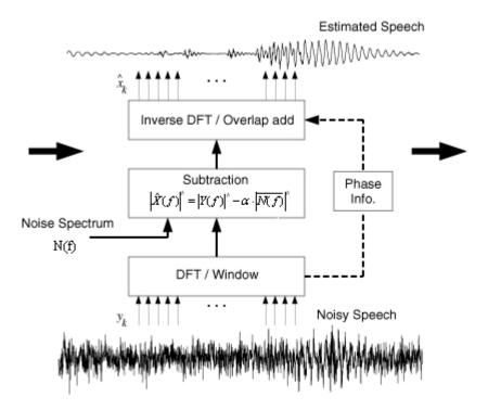
Figure 1: Overview of spectral subtraction method (see \*9)
