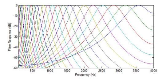
Figure 6: Magnitude response of a 24-band Gammatone filterbank.
