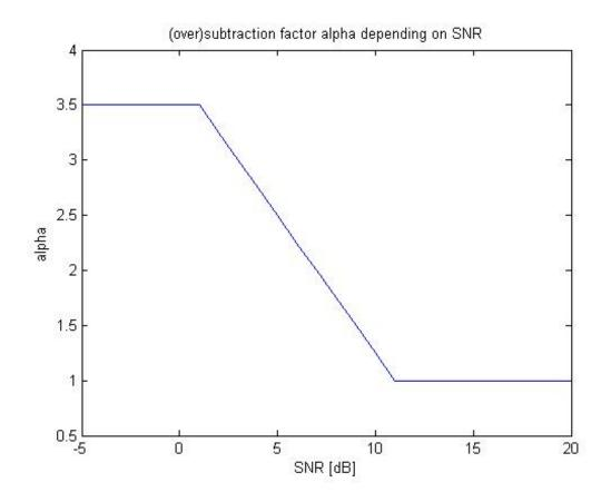
Figure 3: Different values for  $\alpha$  depending on the SNR of the power spectra.
