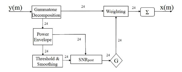
Figure 8: Block diagram of the Gammatone filterbank denoising system.
