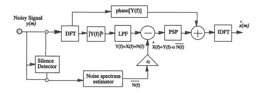
Figure 5: Spectral subtraction in detail
