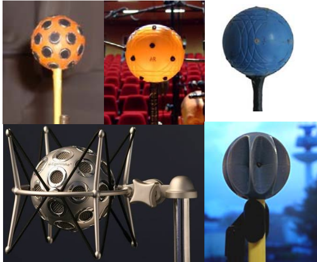
Figure 4 – Some microphone arrays experimented, built by Orange Labs (top, plus "The Sceptre" at bottom-right) except the EigenMike™ from mh-acoustics (bottom-left). Other prototypes are shown in [27]
