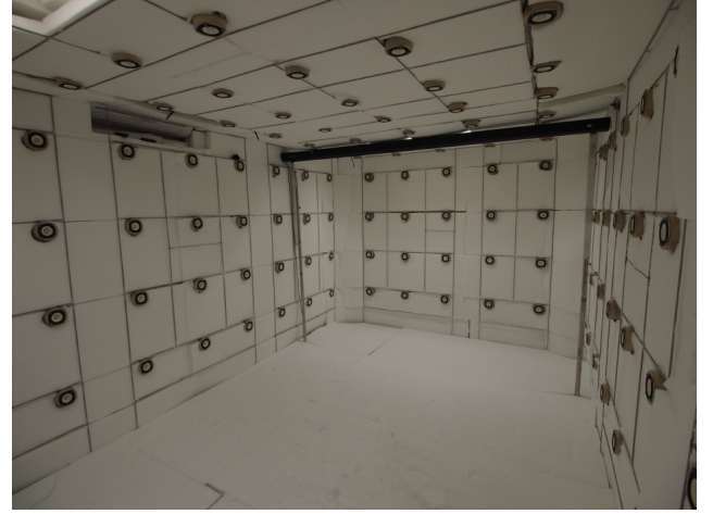
Figure 6: Irregular, 157-channel loudspeaker array inside a semi-anechoic room in the Research Institute of Electrical Communication, Tohoku University.
