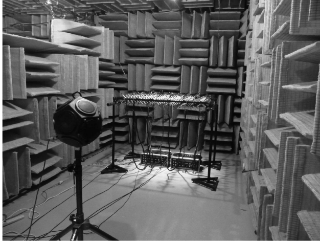
(a) Photography of the experimental setup in the hemi-anechoic room.
