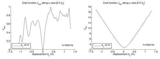
(a)  $J_{ssc}$  cost function for real-valued multipole, (b)  $J_{loc}$  cost function for real-valued multipole,  $N_s = 4$   $N_s = 4$
