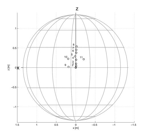
Figure 7.48: Loudspeaker positions found with centering (side-view), exponential sweep measurement, centering frequency 600 Hz
