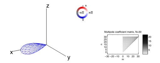
Figure 5.8: Example of a focusing multipole radiation pattern and its spectral distribution
