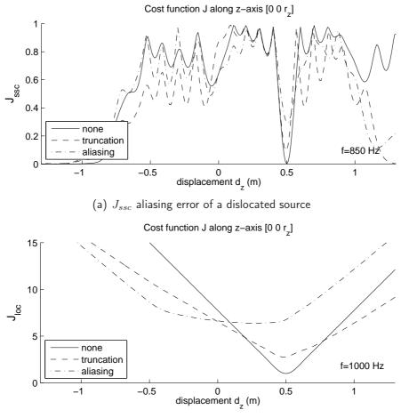
(b)  $J_{loc}$  aliasing error of a dislocated source
