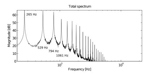
Figure 7.41: Spectrum and partials of trombone playing C4
