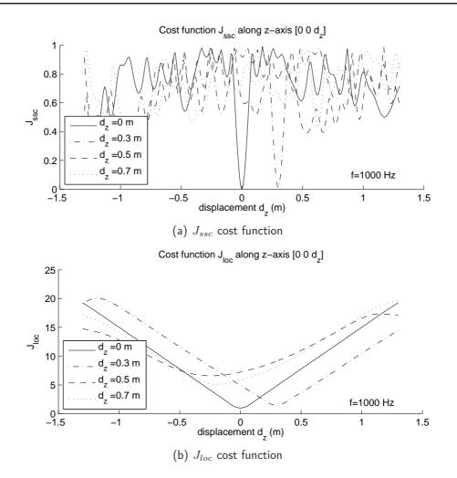
Figure 7.14: Cost functions for different source positions  $a_z$  (centered monopole source at 1000 Hz)
