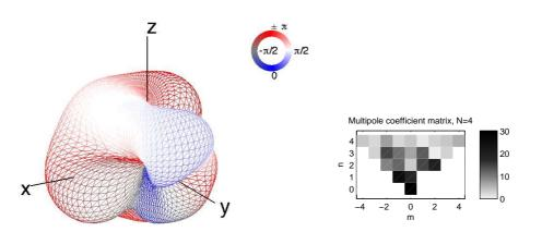
Figure 5.7: Example of a complex-valued multipole radiation pattern with random coefficients and its spectral distribution
