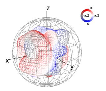
Figure 2.4: Example of a far-field radiation pattern: Trumpet playing A5, observed partial at 888Hz, shown is the extrapolated sound-pressure distribution within a dynamic range of the top 20dB.
