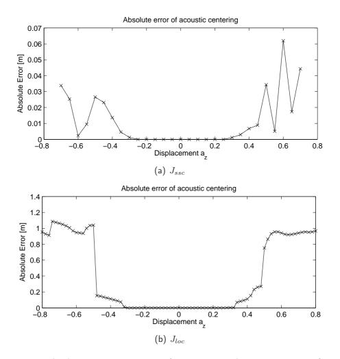
Figure 7.17: Absolute centering error for a monopole source using fminsearch optimization, f = 1000 Hz. Both criteria perform well in the case of a monopole source. A radial bound of confidence can be estimated.
