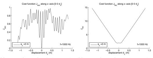
(a)  $J_{ssc}$  cost function for a dipole source along (b)  $J_{loc}$  cost function for a dipole source along z-axis z-axis
