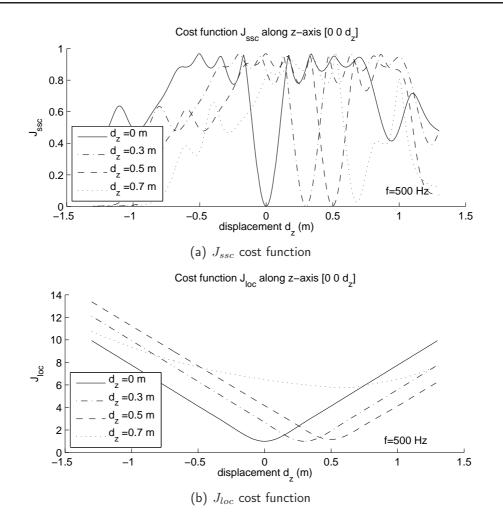
Figure 7.13: Cost functions for different source positions  $a_z$  (centered monopole source at 500 Hz)
