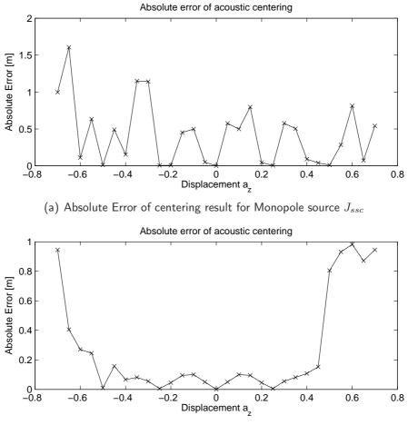
(b) Absolute Error of centering result for Monopole source  $J_{loc}$
