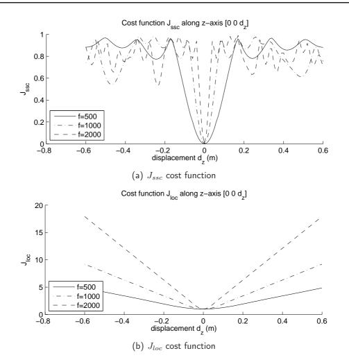
Figure 7.12: Cost functions at different frequencies (centered monopole source)
