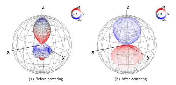
Figure 7.24: Radiation pattern comparison (dipole source dislocated at  $a_z = 0.3m$ , f = 1000Hz). The centering by  $d_{min}$  yields the dipole-like phase distribution.
