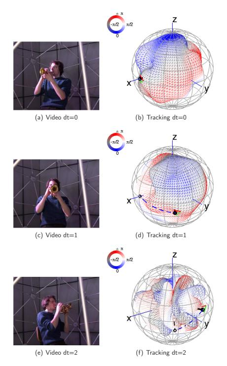
Figure 6.2: Example of rotational tracking, trumpet rotating around z-axis while playing Bb4, partial at 718 Hz
