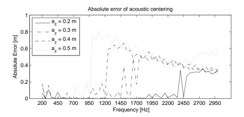
Figure 7.20: Centering error for a monopole source. The upper frequency bound corresponds to the values examined by eq. 5.4 (1893Hz for  $a_z = 0.2m$ , 1263Hz for  $a_z = 0.3m$ , 947Hz for  $a_z = 0.4m$  and 758Hz for  $a_z = 0.5m$ )
