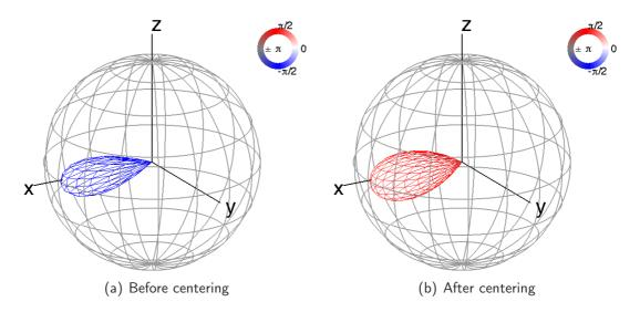
Figure 7.25: Radiation pattern comparison (directional source at the origin, f = 1000Hz). A directional source may be centered by the optimization algorithm even if the source has not been dislocated.
