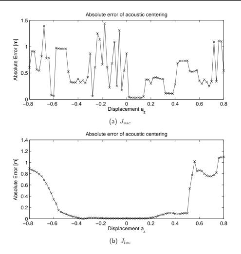
Figure 7.19: Absolute centering error for a complex-valued multipole source, f = 1000Hz. The  $J_{ssc}$  criterion fails throughout all shifts except for a small range. A statistical analysis is assumed to show random results since the phase relations are randomly chosen. The  $J_{loc}$  crierium still performs well in a certain radial bound.
