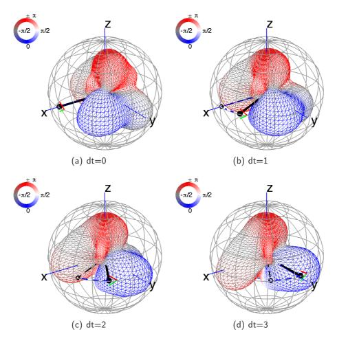
Figure 6.1: Example of rotational tracking, simulated complex valued multipole source rotating around z-axis (f = 1000Hz)
