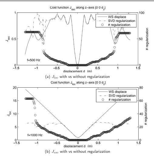
Figure 7.5: Effects on the cost function due to the regularization of the wave spectrum estimation
