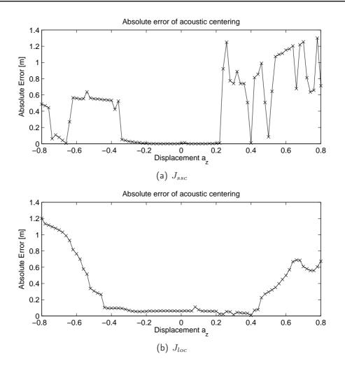
Figure 7.18: Absolute centering error for a real-valued source using fminsearch optimization, f = 1000Hz. In case of  $J_{ssc}$ , the criterion fails at a smaller bound than with a monopole source. An error bias can be observed when using the  $J_{loc}$  cost function, maybe due to the directional sound radiation.
