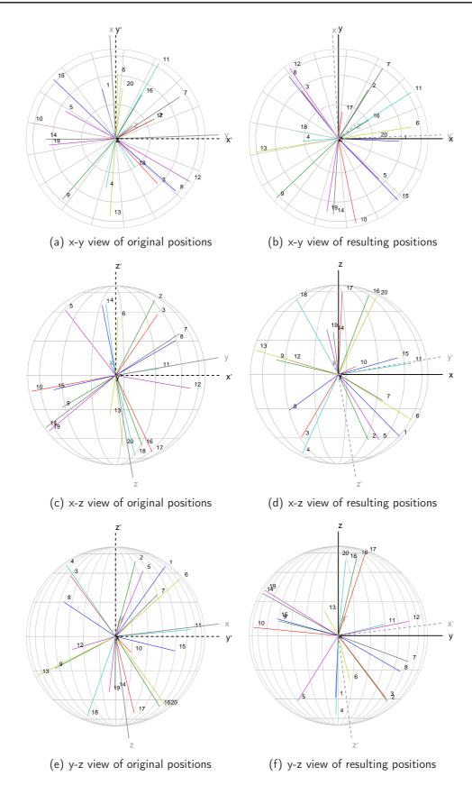
Figure A.2: Example calibration with icosahedron (20 loudspeakers)
