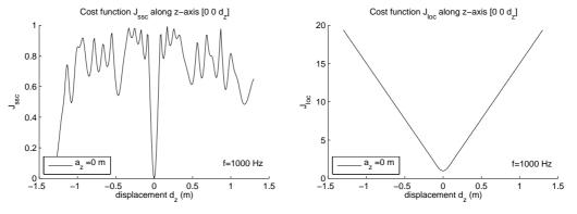
(a)  $J_{ssc}$  cost function for a monopole source (b)  $J_{loc}$  cost function for a monopole source
