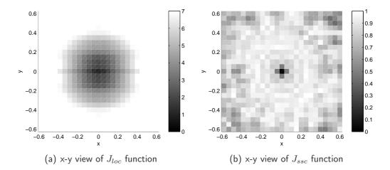
Figure 7.15: Example localization map - centered monopole source, slice at z = 0
