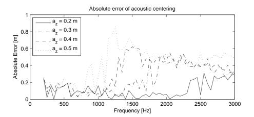
Figure 7.22: Centering error for a complex-valued multipole source of order  $N_{mult} = 4$ . The result is similar to the case of a real-valued multipole as expected. However, the error seems to be more arbitrary
