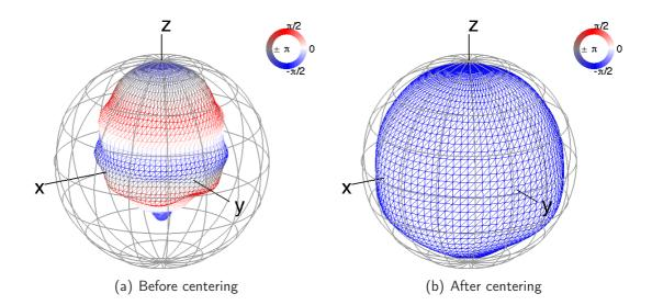
Figure 7.23: Radiation pattern comparison (monopole source dislocated at  $a_z = 0.3m$ , f = 1000Hz). The centering by  $-d_{min}$  yields a coherent phase distribution on the surface.
