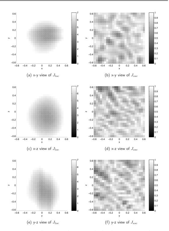
Figure 7.38: Cello, C4, partial at 788 Hz, sliced at (0.13, -0.01, -0.17)m
