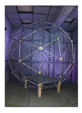
Figure 3.1: Picture of the surrounding spherical microphone array at IEM Graz, Austria
