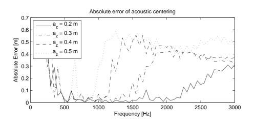
Figure 7.21: Centering error for a real-valued multipole source of order  $N_{mult} = 4$ . Corresponding to eq. 5.4, the frequency bound is assumed to fall due to higher-order components of the source. However, the strong increase of the error stays at the bounds of the above plot
