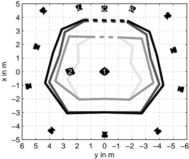
**Figure 4:** Median sweet spot radius for each loudspeaker direction except C. Gray levels indicate conditions: light gray - 1<sup>st</sup>-order original, gray - 1<sup>st</sup>-order SDM, dark gray - 3<sup>rd</sup>-order SDM, black - 5<sup>th</sup>-order SDM.
