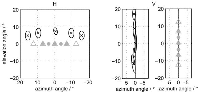
**Figure 2:** Mean (×) and 95% confidence areas (○) of localization and energy vector (Δ) and velocity vector (●) for array H and V.
