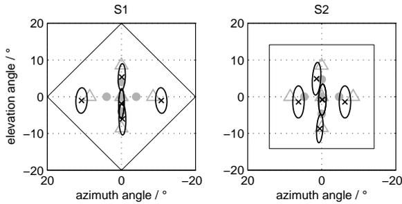
**Figure 6:** Mean (×) and 95% confidence areas (○) of localization and energy vector (Δ) and velocity vector (●) for array Q1 and Q2.
