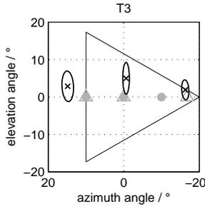
**Figure 5:** Mean (×) and 95% confidence areas (○) of localization and energy vector (Δ) and velocity vector (●) for array T3.
