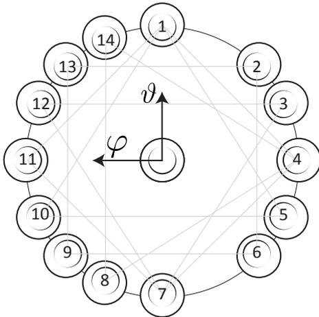
**Figure 1:** Sketch of the loudspeaker setup with implied loudspeaker arrays.
