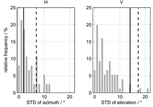
**Figure 3:** Histogram of the intrasubjective standard deviation (■) compared to the median of the intersubjective standard deviation (–) and the total standard deviation of all conditions and answers (– –) tested with array H and V.
