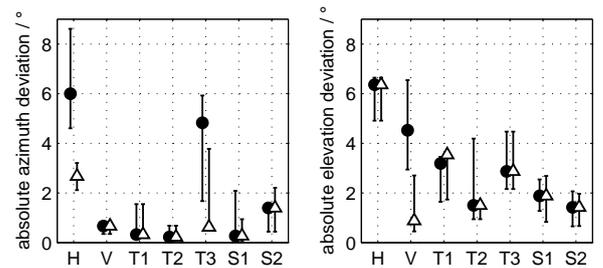
**Figure 7:** Median and 95% confidence interval of the absolute azimuth and elevation deviation of the velocity vector (●) and energy vector (Δ) from the mean experimental results for each array.
