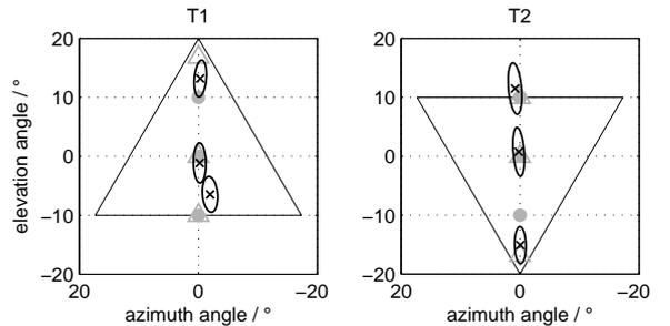
**Figure 4:** Mean (×) and 95% confidence areas (○) of localization and energy vector (Δ) and velocity vector (●) for array T1 and T2.
